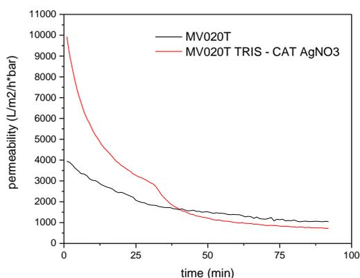
Picture 3. Water permeability for pristine and modified membrane MV020T.
