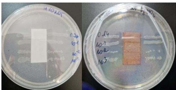
Picture 2. Antibacterial test with AATCC method 147 for pristine MV020T (left) and modified membrane (right).
