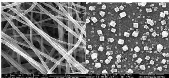
Picture 1. Imbedded AgNPs on the nanofibers PA PVDF membrane (left) and MV020T membrane (right).
