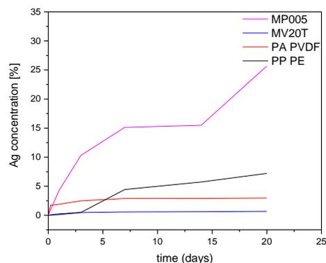
Picture 4. The percent of released AgNPs during filtration for each modified membrane.
